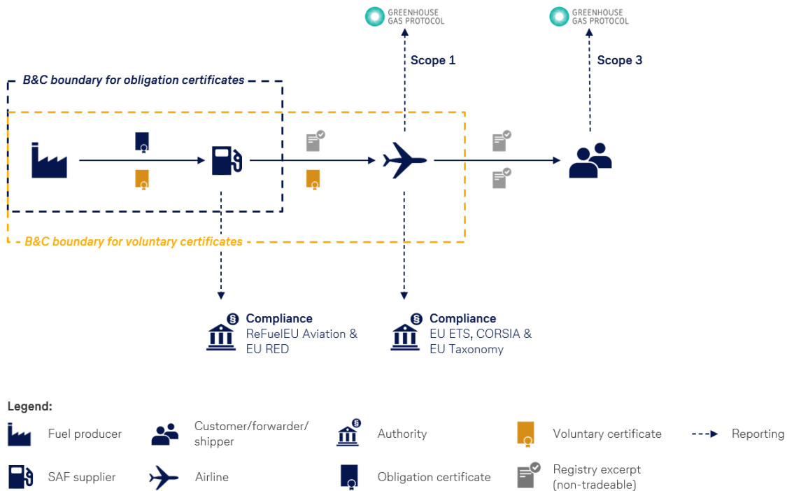
Figure 3: Design of the proposed SAF book-and-claim system (yellow: balance boundary).
